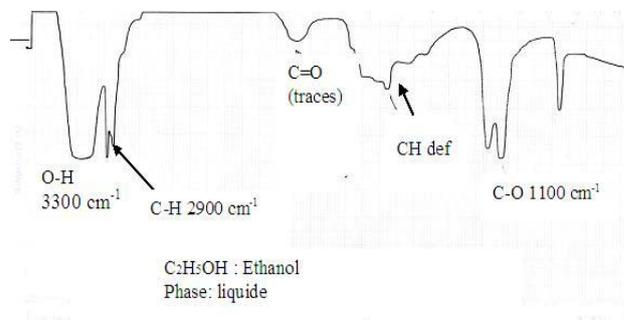
Fig. 7 Infrared spectrum of the final product
