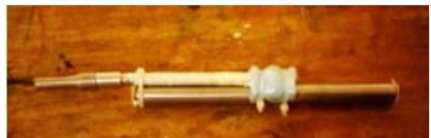
Fig. 2 Thermocouple J type, attached to the cylindrical probe
