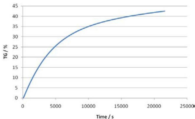
Fig. 1b CH<sub>4</sub> decomposition at 850 °C
