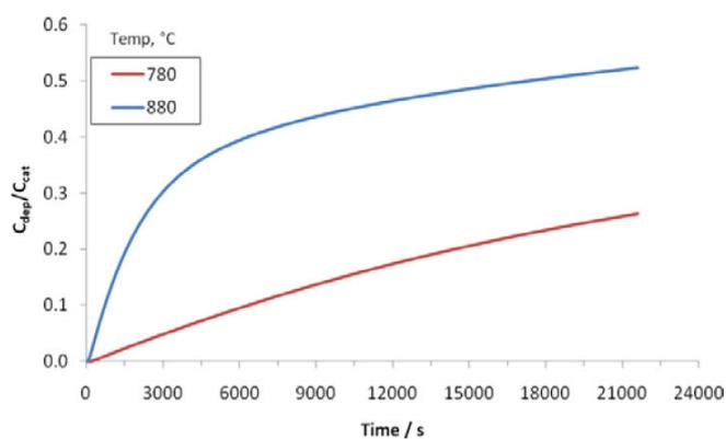
Fig. 2a Carbon mass gain at 50 vol.% methane
