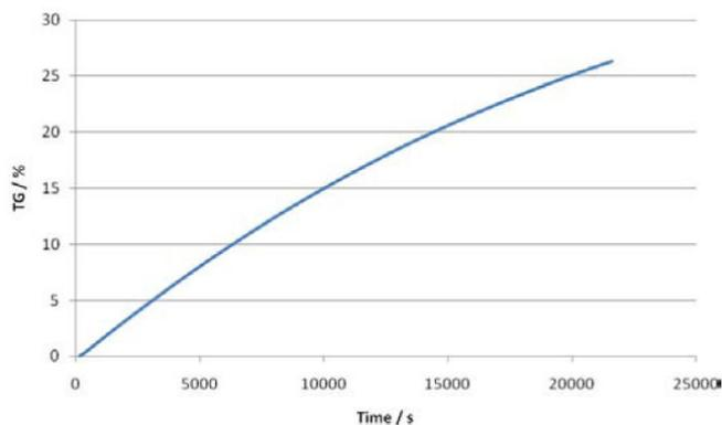
Fig. 1a CH<sub>4</sub> decomposition at 780 °C
