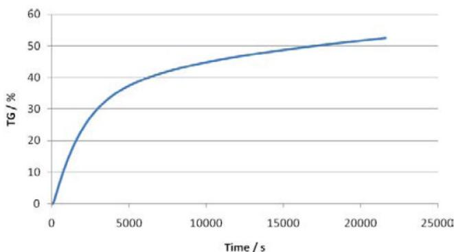
Fig. 1c CH<sub>4</sub> decomposition at 880 °C
