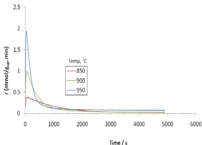
Fig. 3b Rate of carbon formation vs time for different temperatures at methane volume percent 25%
