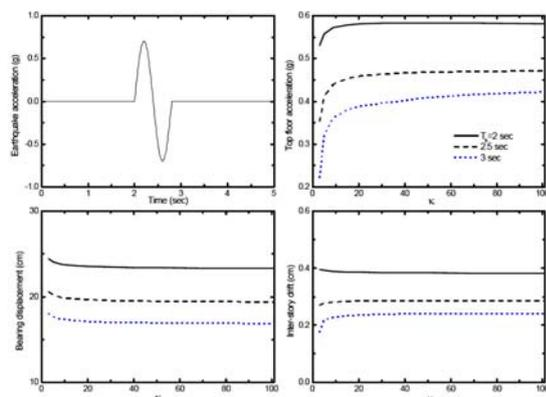
Fig. 11. Variation of the top floor acceleration, middle-story drift and the bearing displacement against the stiffness ratio,  $\kappa$  under the pulse associated in Imperial Valley, 1979 earthquake recorded at Array # 5 ( $\mu = 0.05$ ).
