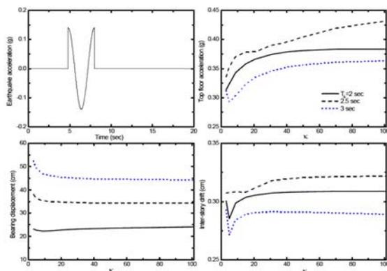
Fig. 12. Variation of the top floor acceleration, middle-story drift and the bearing displacement against the stiffness ratio,  $\kappa$  under the pulse associated in Northridge, 1994 earthquake recorded at Rinaldi station ( $\mu = 0.05$ ).
