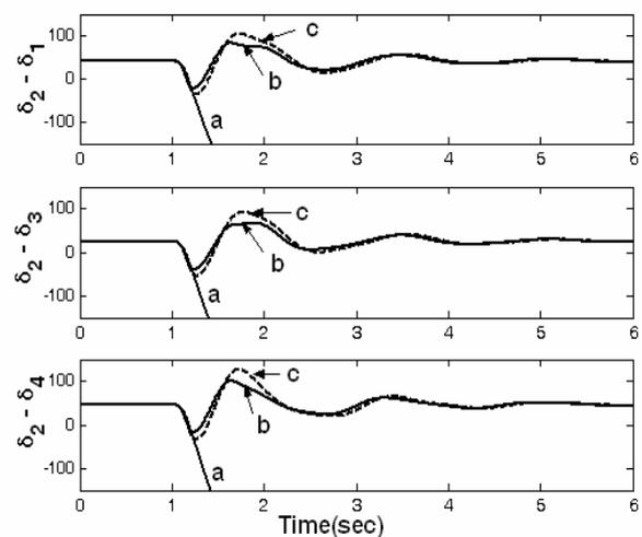
Fig. 8 Relative rotor angles following a 3 phase fault at bus 2 for 0.1 sec with (a) no control, (b) PSO based loop-shaping control, and (c) graphical loop shaping control.
