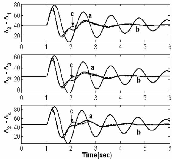
Fig. 7 Comparison of relative angles for a 50% input torque pulse on generator 2 for 0.1s with (a) no control, (b) PSO based loop-shaping, and (c) graphical loop-shaping
