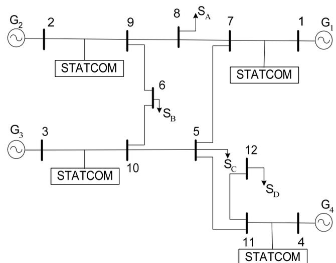
Fig. 1 A 4-machine power system with STATCOM
