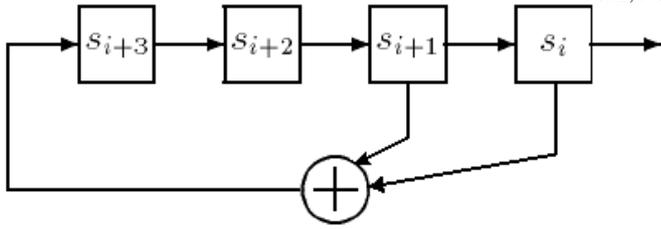
Fig. 1. The additive shift register structure.
