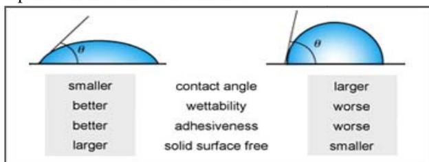
Fig. 13 Comparison between smaller and larger contact angle
