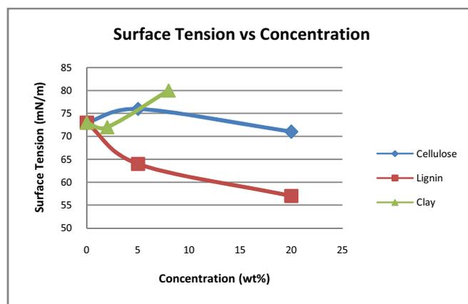
Fig. 2 Surface Tension for different concentration of biomass
