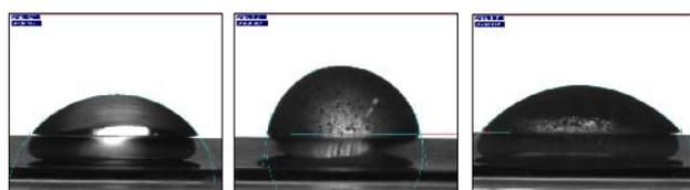
Fig. 3 Sessile drop images for (a) 0% cellulose, (b) 5% cellulose (c) 20% cellulose onto glass surface
