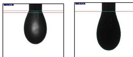
Fig. 11 Pendant drop images for (a) 5% lignin, (b) 20% lignin
