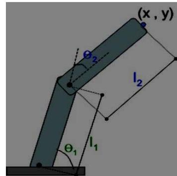
Fig. 6 End effector's coordinates of a manipulator
