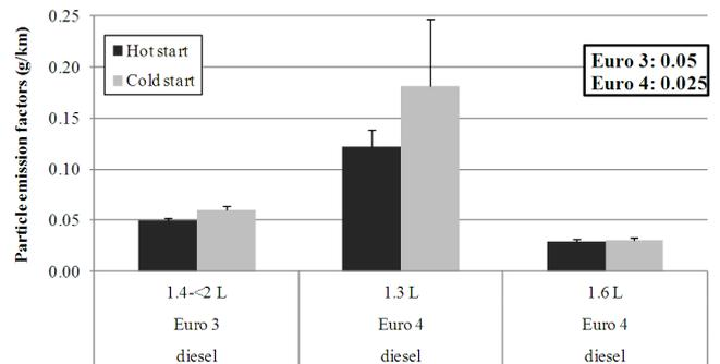
Fig. 3 Average particle emissions on the ARTEMIS Urban driving cycles for some of the diesel vehicles and comparison with European emission standards
