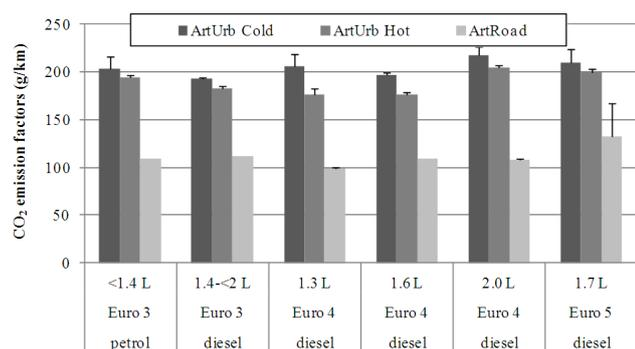
Fig. 5 Average CO<sub>2</sub> emissions for some of the vehicles, under different ARTEMIS driving cycles
