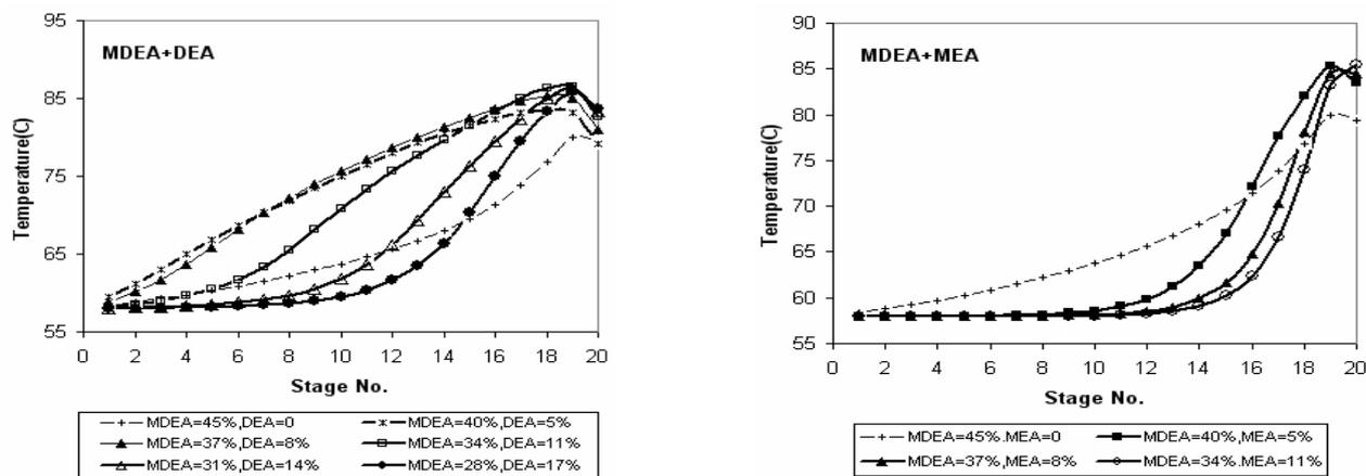
Fig. 2. Effect of amine mixture on absorber temperature
