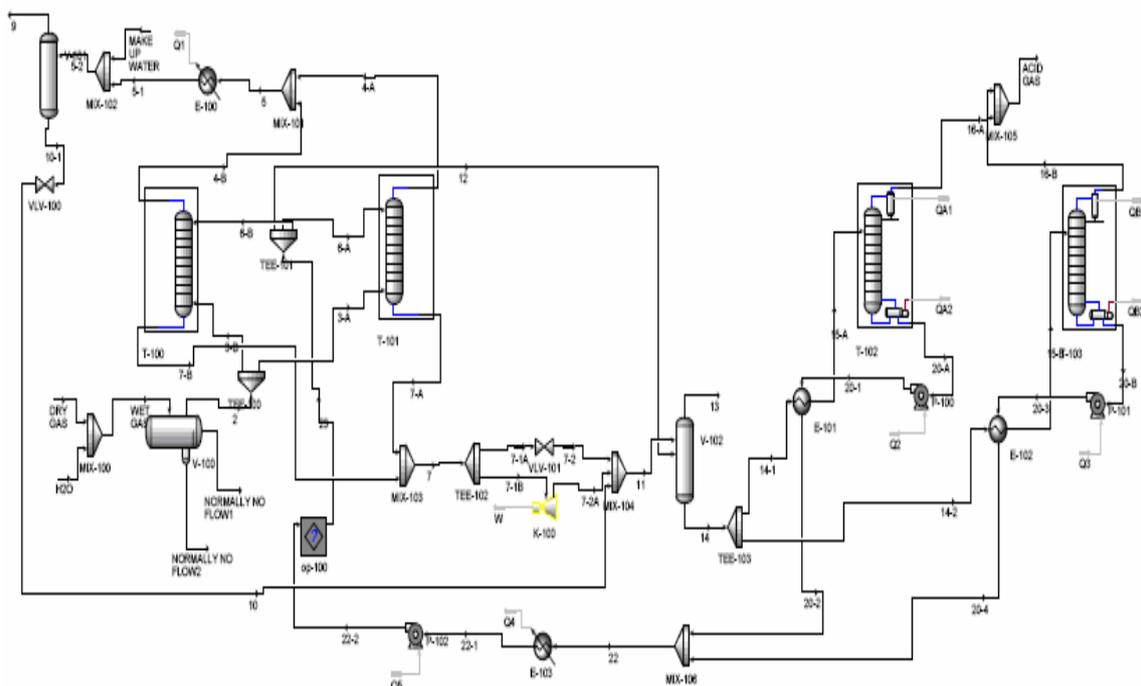
Fig. 1. Schematic of gas sweetening process by HYSYS
