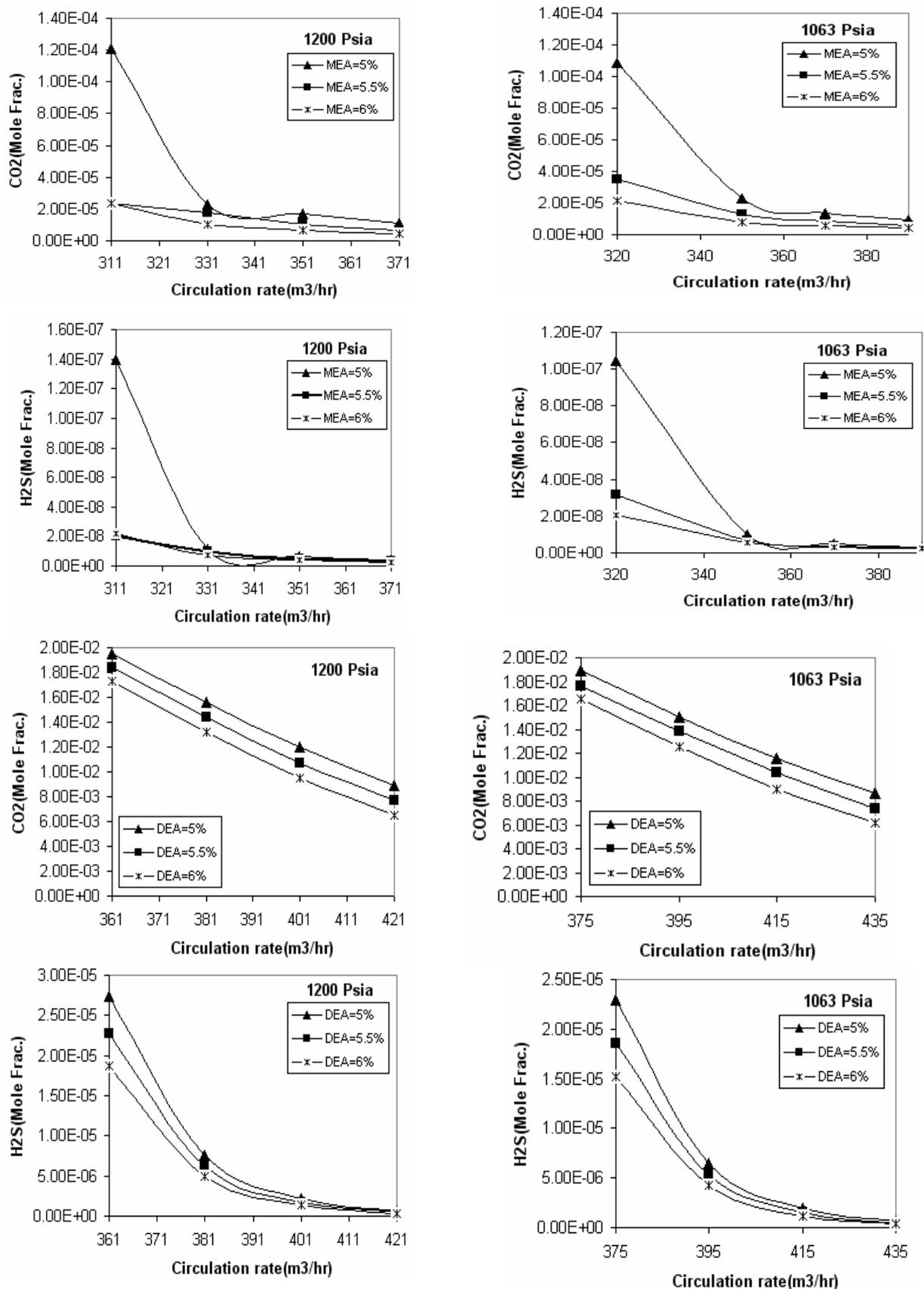
Fig. 4. Effect of pressure on amine mixture
