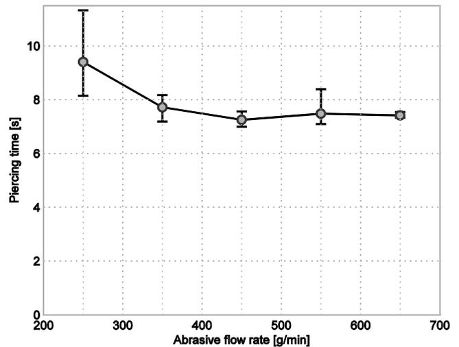
Fig. 6 Piercing time as a function of abrasive flow rate
