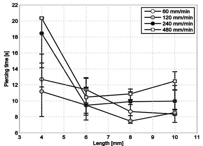
Fig. 9 Piercing time as a function of path length of repeated linear piercing
