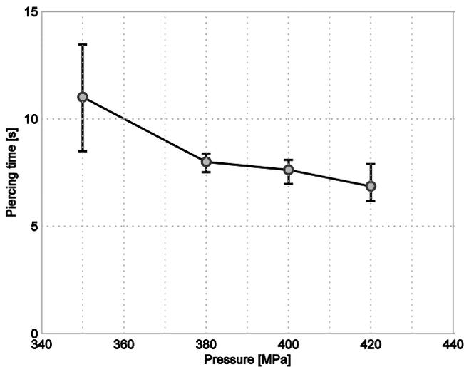
Fig. 4 Effect of water pressure on piercing time
