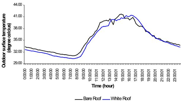
Fig. 7 (c) Comparison of outdoor surface temperature between bare roof and white roof for six days' reading
