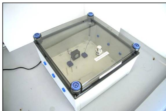
Fig. 3 The low volume environmental testing chamber
