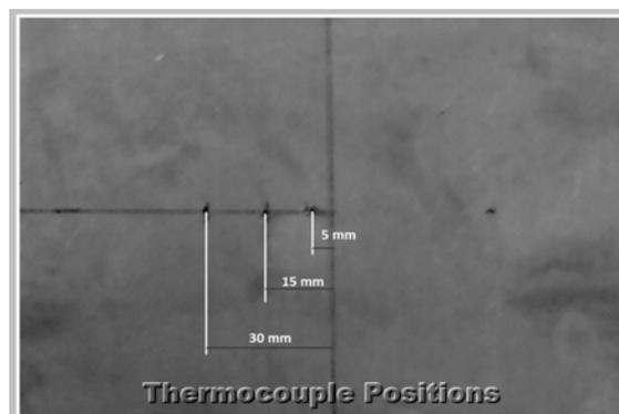
Fig. 2 Thermocouple positions
