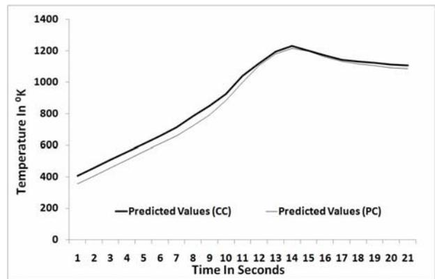
Fig. 9. Predicted values of temperature at weld centre
