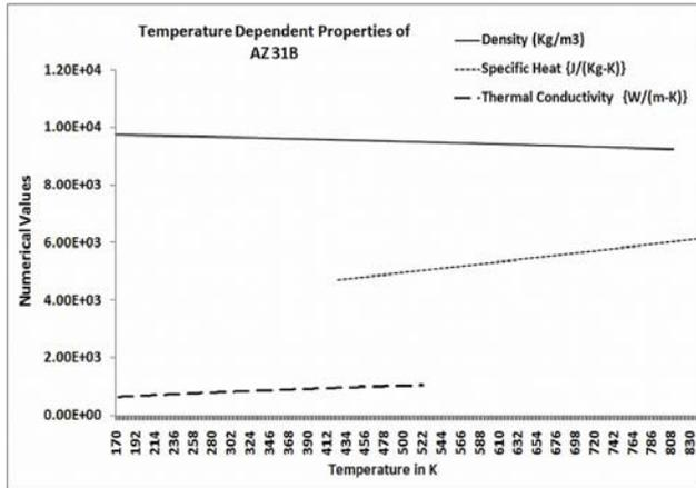
Fig. 3. Temperature dependent properties of AZ31 B
