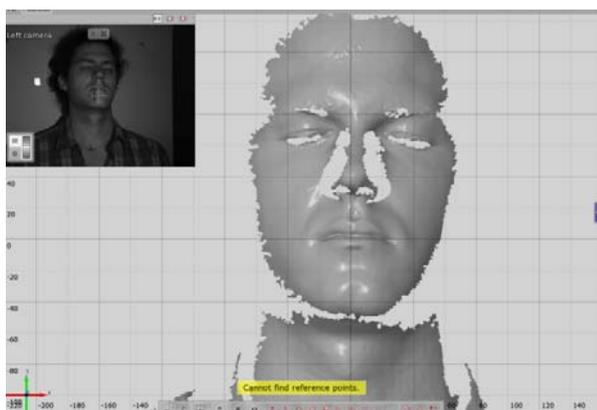
Fig. 10 ATOS I without reference points, 1 snapshot
