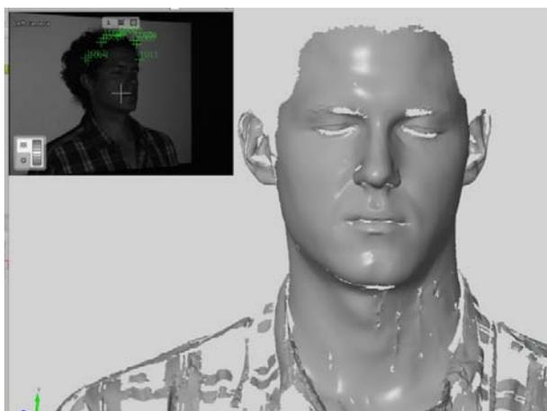
Fig. 14 ATOS Triple scan with headband, 3 snapshots
