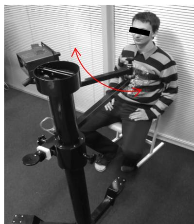
Fig. 9 Stand with swinging arm for ATOS I
