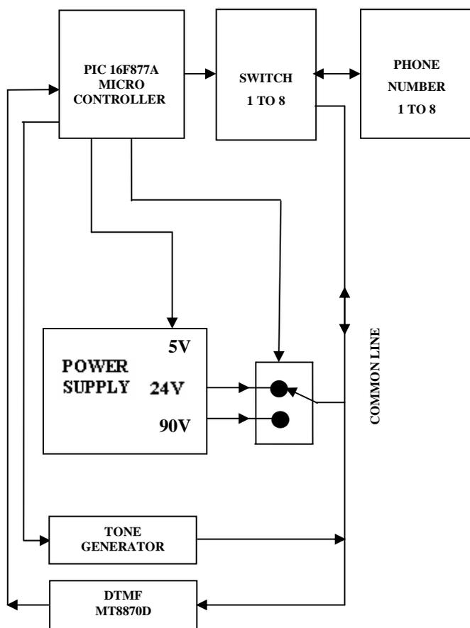
Fig. 1 Block Diagram of Microcontroller-Based Telephone Exchange
