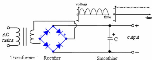
Fig. 2 Output Voltage of a Power Supply
