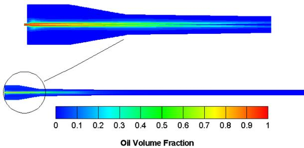
Fig. 5 Distribution of oil in deoiling hydrocyclone
