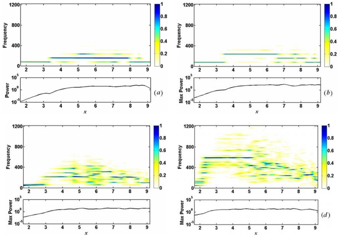
Fig. 6 Spectra of average horizontal convection  $H(x)$  normalized by the maximum power of each  $x$  position for different Rayleigh numbers. (a)  $Ra = 1.4 \times 10^6$  (b)  $Ra = 2.1 \times 10^6$  (c)  $Ra = 3.5 \times 10^6$  (d)  $Ra = 1.4 \times 10^7$
