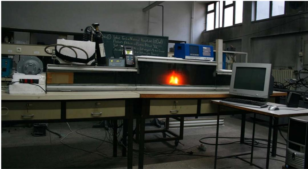
Fig. 1 Photograph of model underground station
