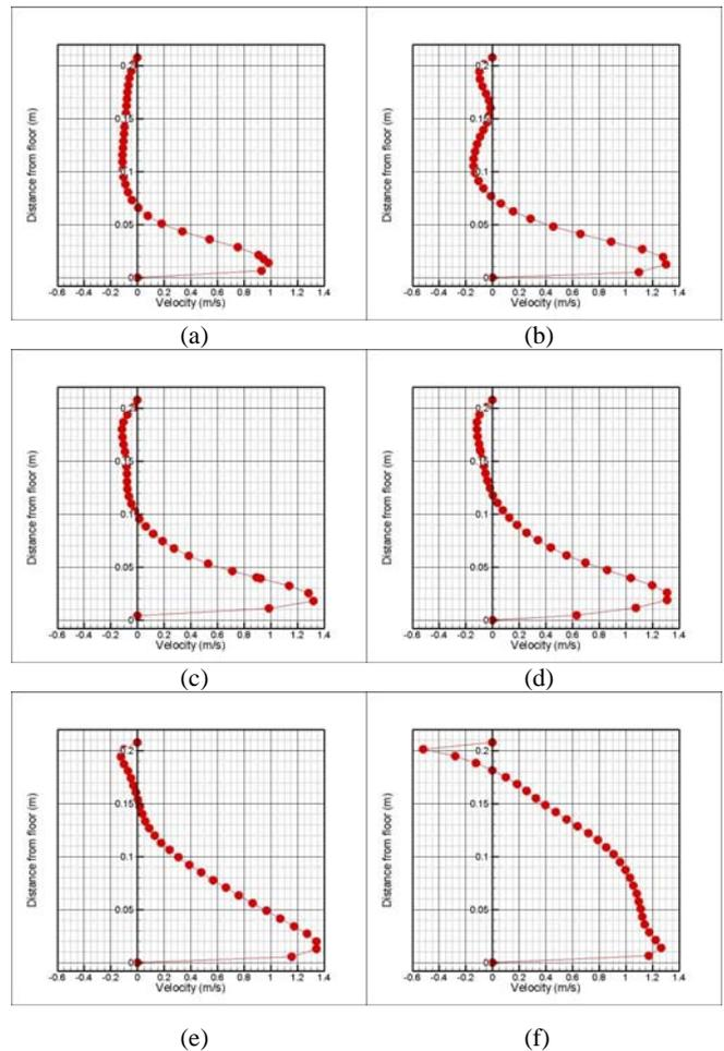
Fig. 9 CFD predicted velocity profiles on the centerline of fuel source at  $t=13$  s for various locations in the station ( $Q=2$  kW  $V_c=1.41$  m/s,  $V_{inlet}=1$  m/s) a) distance from station entrance is 10 cm, b) distance from station entrance is 25 cm, c) distance from station entrance is 40 cm, d) distance from station entrance is 50 cm, e) distance from station entrance is 60 cm, f) distance from station entrance is 70 cm
