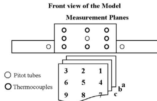
Fig. 3 Locations of thermocouples and pitot tubes
