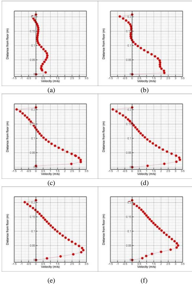
Fig. 10 CFD predicted velocity profiles on the centerline of fuel source at  $t=13$  s for various locations in the station ( $Q=2.3$  kW  $V_c=1.47$  m/s,  $V_{inlet}=3$  m/s) a) distance from station entrance is 10 cm, b) distance from station entrance is 25 cm, c) distance from station entrance is 40 cm, d) distance from station entrance is 50 cm, e) distance from station entrance is 60 cm, f) distance from station entrance is 70 cm
