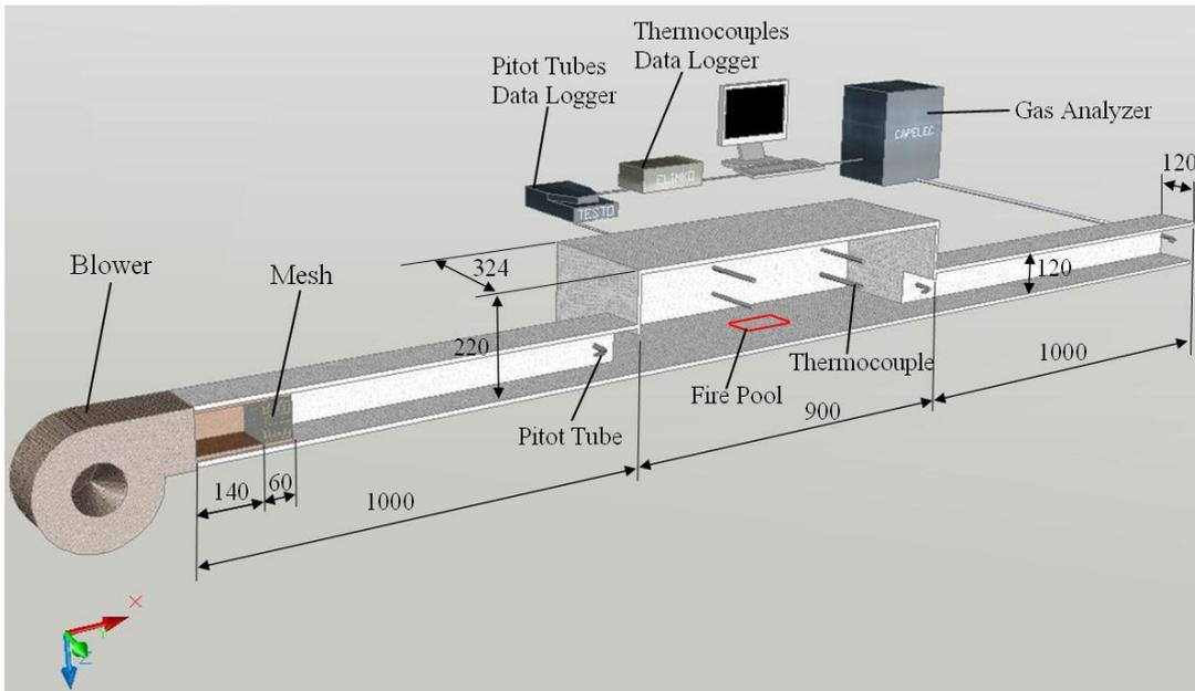
Fig. 2 Schematic diagram of model underground station
