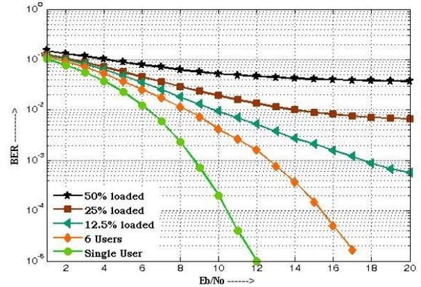
Fig. 5. BER plot of DS-CDMA system using RNS based PN sequence with  $\beta = 64$  for different loading scenarios
