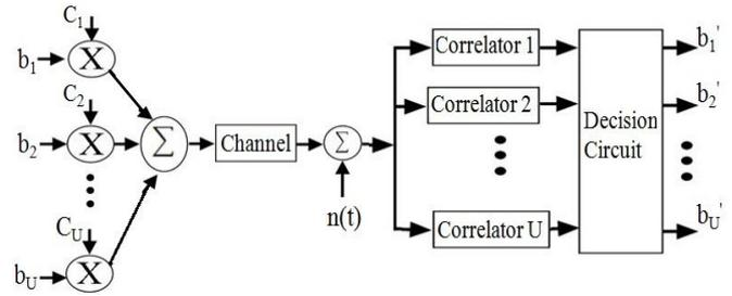
Fig. 1. Block Diagram of DS-CDMA System
