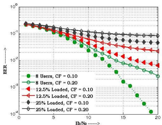
Fig. 10. BER Performance of DS-CDMA system using RNS based PN sequence with  $\beta = 128$  for different loading scenarios. The channel considered is Rayleigh Fading Channel with cross-correlation threshold, CF, 0.20 and 0.10
