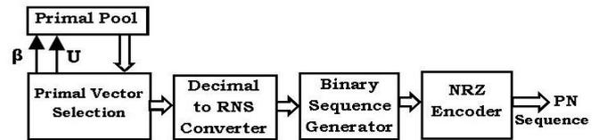
Fig. 3. RNS Based PN Sequence Generation - On-line Process
