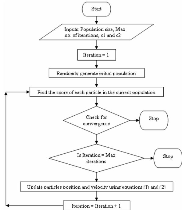
Fig. 2 Flow chart of particle swarm optimization
