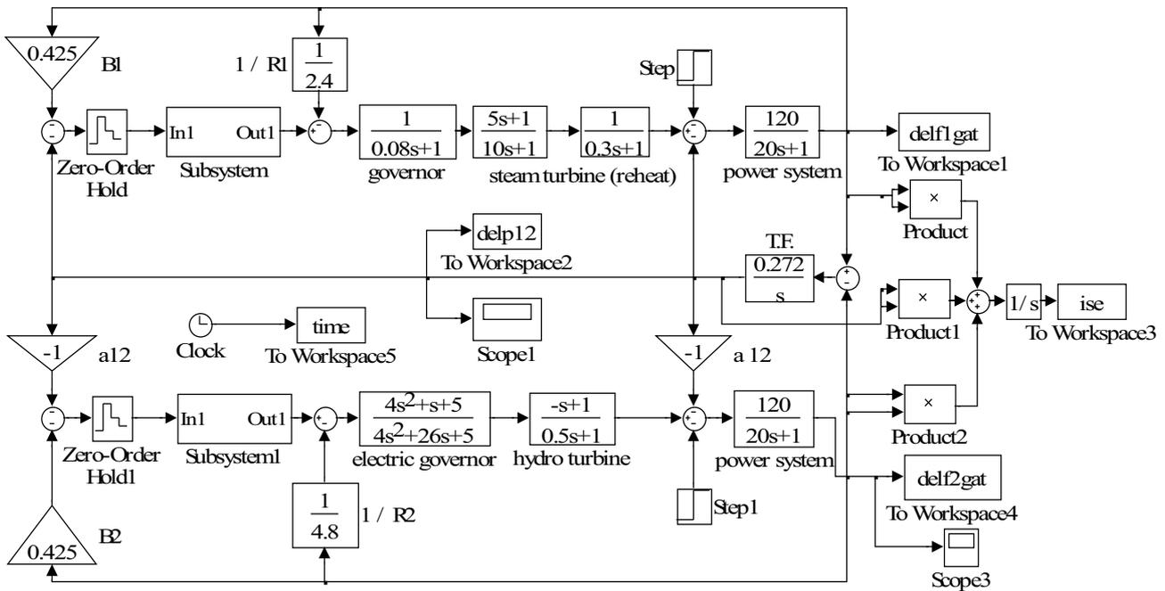
Fig. 7 MATLAB® model of the interconnected hydrothermal system
