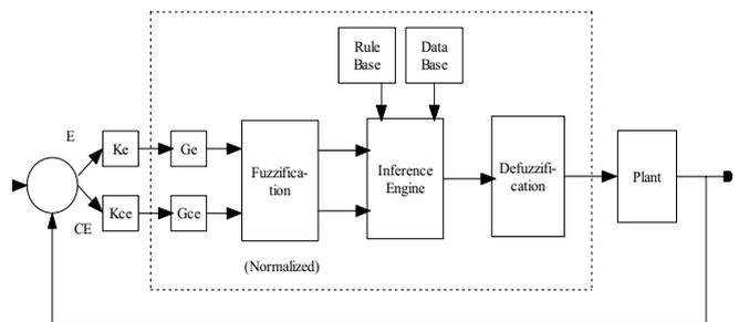
Fig. 5 Tuning parameters for input scaling factors
