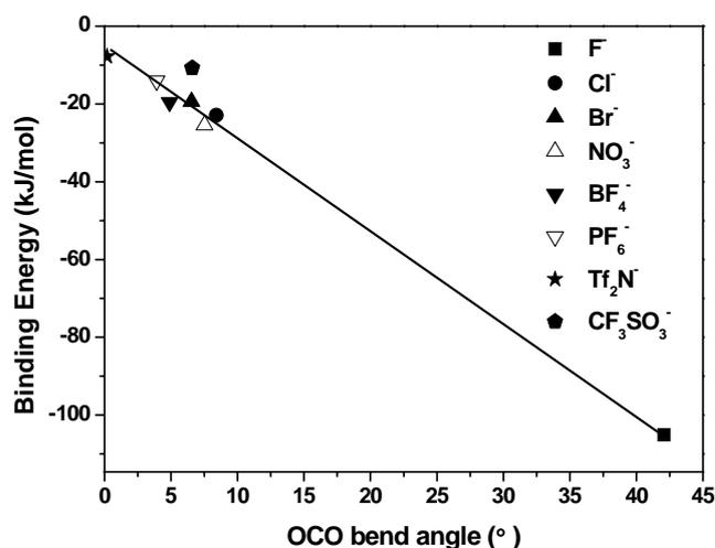
Fig. 3 Binding energy of anion-CO<sub>2</sub> dimer versus deviation of OCO angle of CO<sub>2</sub> molecule from 180° in various complexes. The dots represent various anions. The continuous line is the best fit to the data
