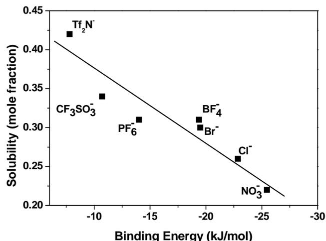
Fig. 4 Comparison of experimentally measured solubility of CO<sub>2</sub> in ionic liquids of different anions containing the same cation (bmim) with binding energy of corresponding complex
