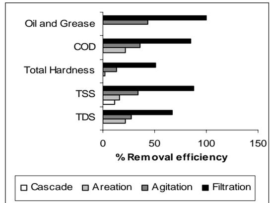
Fig. 7 % Removal efficiency of gray water pollutant in each stage of plant at 2.5 LPM water flow rate
