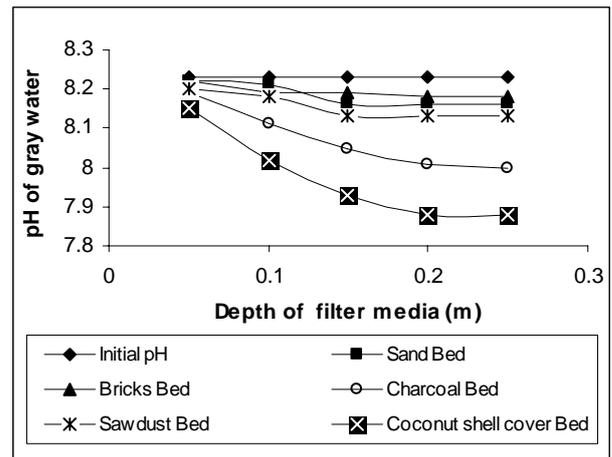
Fig. 2 Effects of filter bed heights on pH level change
