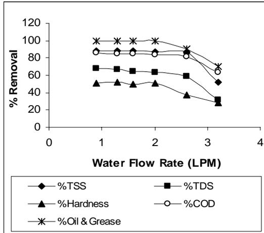
Fig. 4 % removal of pollutants with water flow rate
