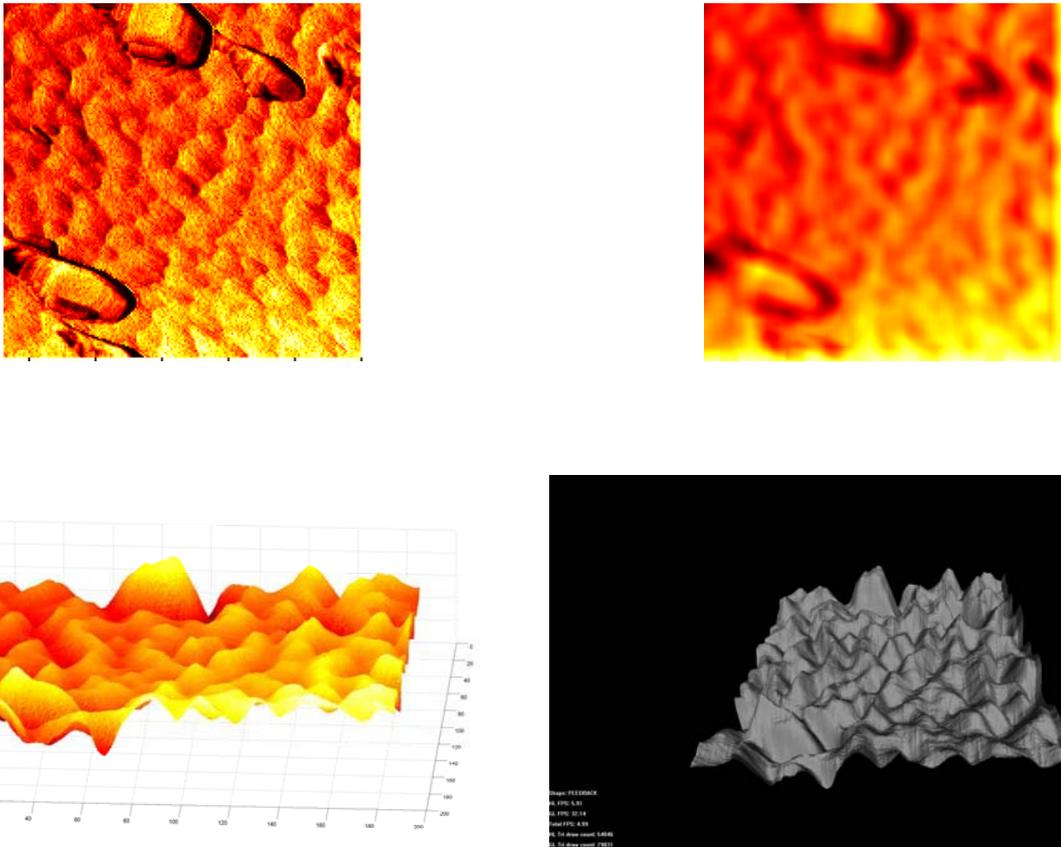
Fig. 6. top-left: Raw AFM image of the scanned sample, top-right: Filtered version of raw Image (left), Bottom-left: Rendered surface of the ltered image (top-right), Bottom-right: Generated virtual Haptics surface
