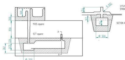
Fig. 2 Schematic diagram of single fluidity test mould [12]
