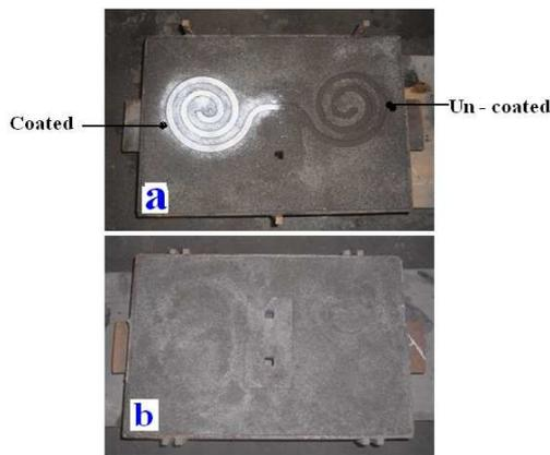
Fig. 3 Green sand moulds made to investigate the fluidity
