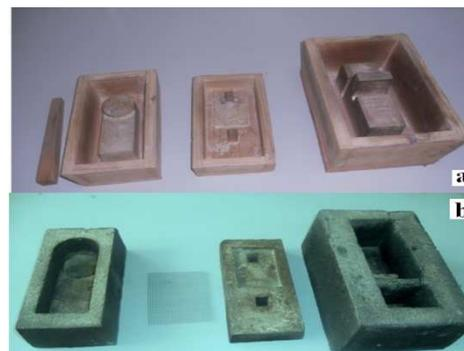
Fig. 1 a) Left to right –sprue, bottom runner core box, top runner core box, pouring basin core box, b) Left to right – Bottom runner core, metal screen, top runner core, pouring basin core
