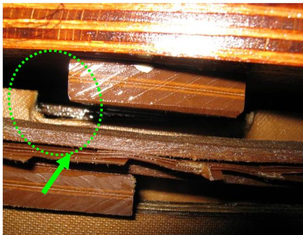
Fig. 8(b): Damaged pressboard due to coaxial force
