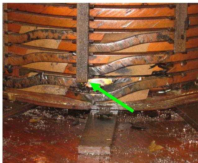
Fig. 12: Arrow shows the arcing spot
