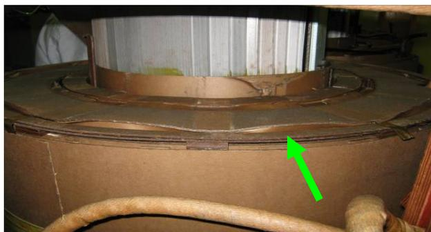
Fig. 9: Wavy pressboard
