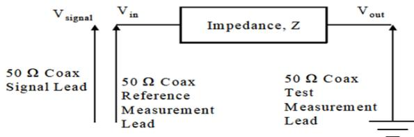
Fig. 2 Test setup for SFRA testing
