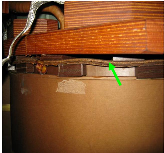
Fig. 8(a): Wavy pressboard due to coaxial force
