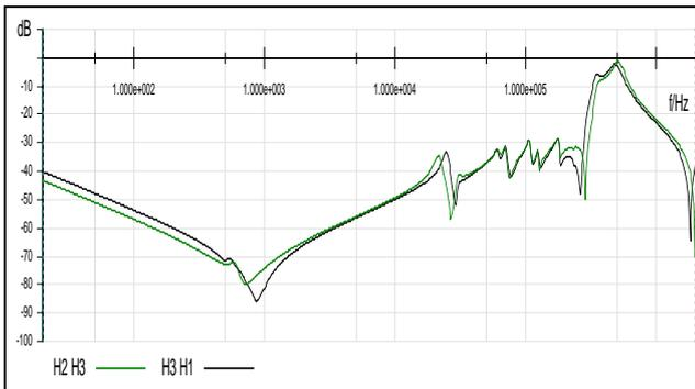
Fig. 7 SFRA results for Y-B and B-R windings (HV)
