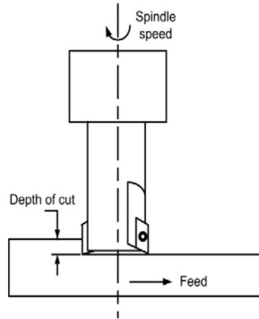
Fig. 1 (b) End Milling – Work-tool motion
