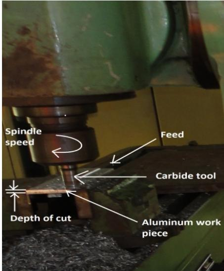
Fig. 1 (a) End Milling – Machining process
