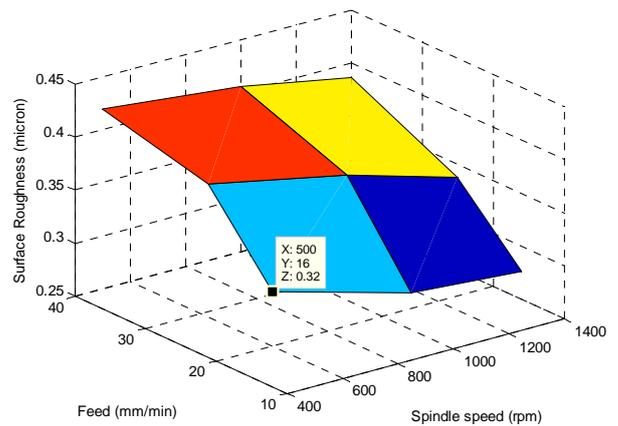
Fig. 2 Surface plot of ‘spindle speed’ and ‘feed’
