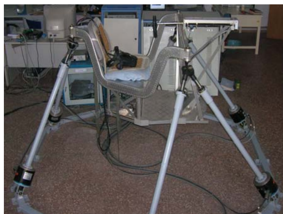
Fig. 1 The parallel motion platform with subsided cabin
