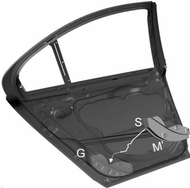
Fig. 15 Path Planning is carried out for the shrunk SIPS unit
