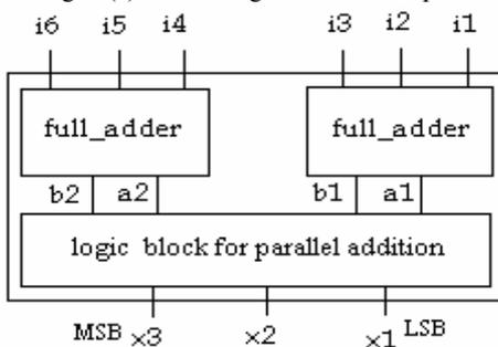
Fig. 6 (b) Block diagram of 6-3 compressor
