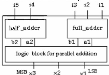
Fig. 6 (a) Block diagram of 5-3 compressor
