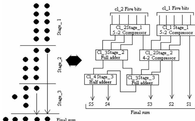
Fig. 8 Bit reduction technique using conventional compressors
