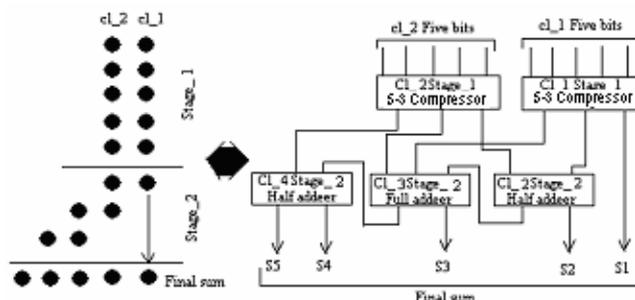
Fig. 9 Bit reduction technique using our compressors
