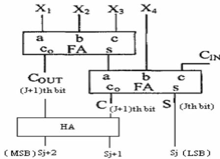
Fig. 2 Modified 4-2 compressor
