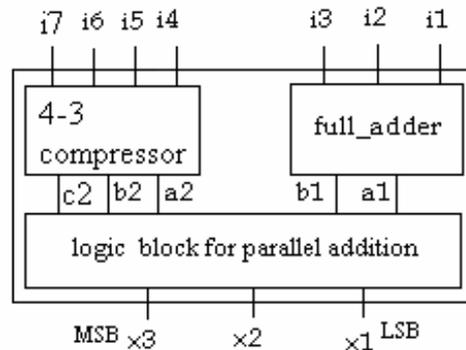
Fig. 6 © Block diagram of 7-3 compressor
