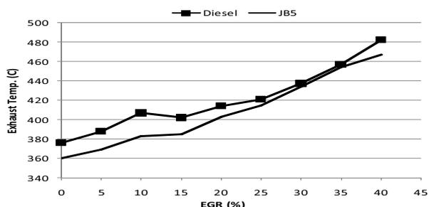
Fig. 6 Variation of exhaust temperature with EGR rates
