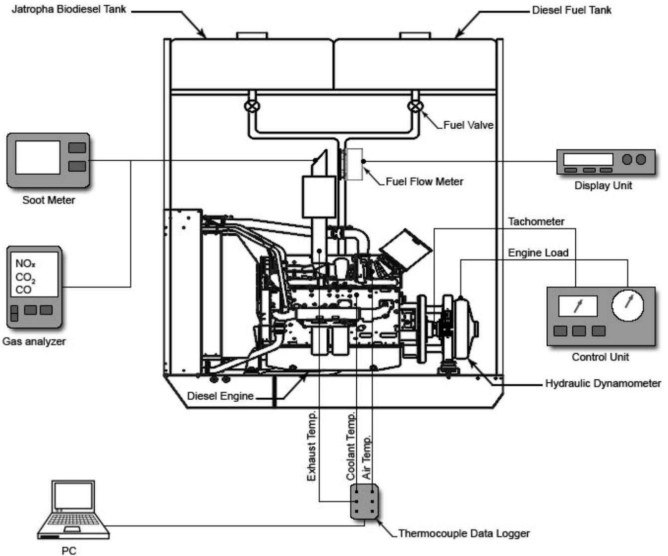
Fig. 1 Experimental setup diagram
