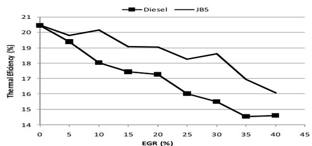
Fig. 3 Variation of thermal efficiency with EGR rates
