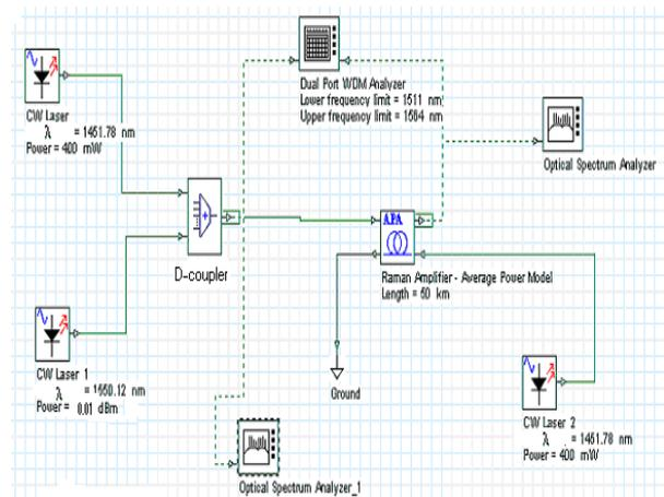
Fig. 2 The simulation layout, bidirectional pumping
