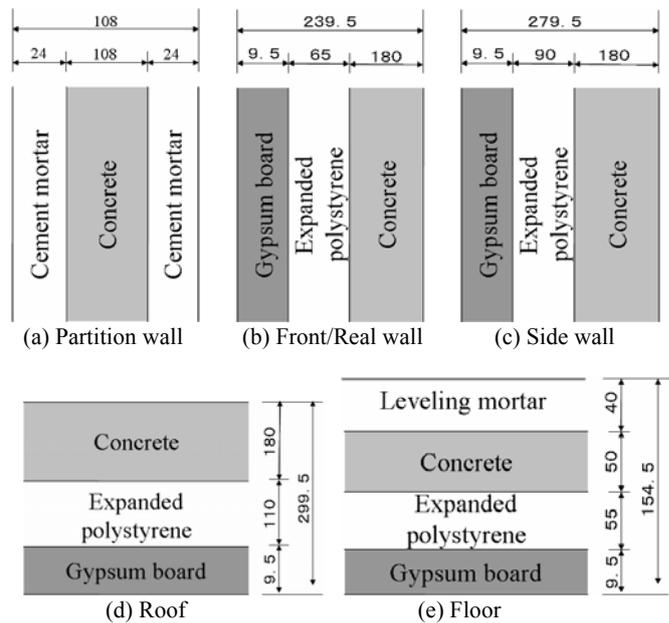
Fig. 4 Details of floors and walls (unit: mm)
