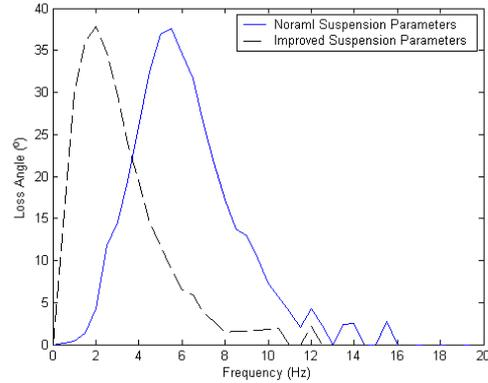
Fig. 21 Loss Angle of air spring response
