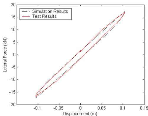
Fig. 11 Hysteresis loop of the air spring in lateral direction,
