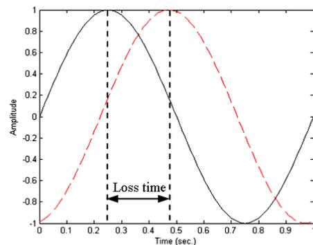
$$D_{Loss\ Angle} = 2\pi f T_{Loss\ time}$$
