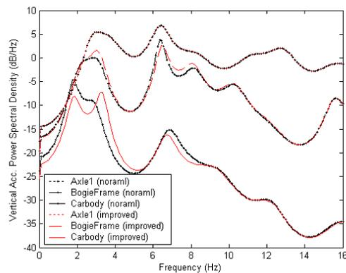
Fig. 22 PSD diagram of accelerations
