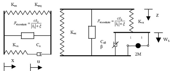
Fig. 5 Proposed modified model for air spring
