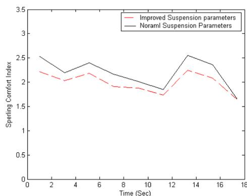
Fig. 23 Spurling ride comfort index for Tehran-Ghazvin route (Straight section) with 80 km/h speed
