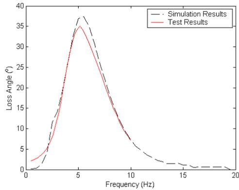
Fig. 9 Loss angle of air spring -  $M = 198.385 \text{ kg}$ ,
