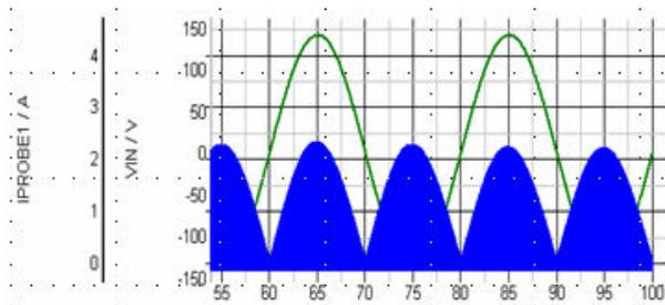
Fig. 19 Input voltage and inductor current.
