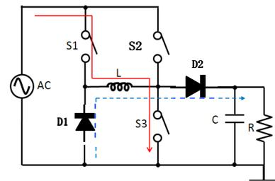
Fig. 1 H-Bridge AC-DC converter (Current when  $V_{in} > 0$ )
