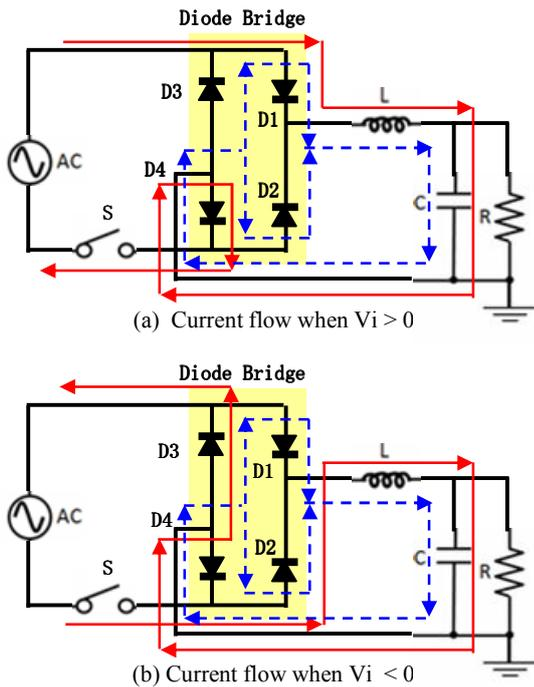
Fig. 10 Direct Buck AC-DC converter
