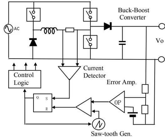
Fig. 16 New BCM PFC without an analog multiplier
