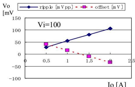
Fig. 21 Output ripple and offset vs. output current
