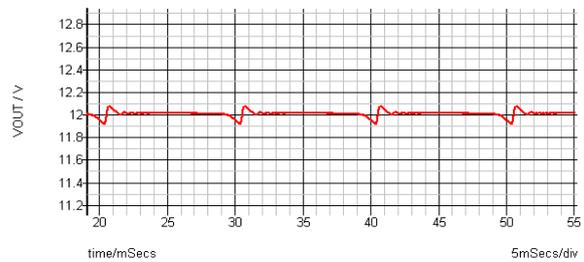
Fig. 12 Output ripple of the inverting converter
