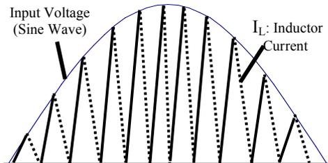
Fig. 15 Waveform of inductor current in BCM
