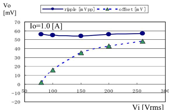
Fig. 22 Output ripple and offset vs. input voltage
