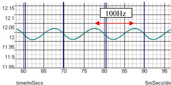
Fig. 18 Output voltage ripple ( $I_o=1.0$  A).
