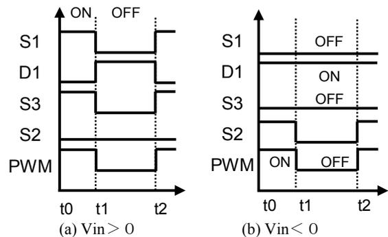
Fig. 3 Timing chart of switches
