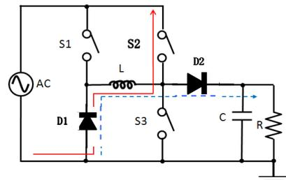
Fig. 2 H-Bridge AC-DC converter (Current when  $V_{in} < 0$ )
