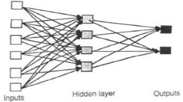
Fig. 5 An example of a multilayered perceptron [8]
