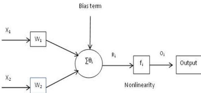
Fig. 4 An example model of a single perceptron [12]
