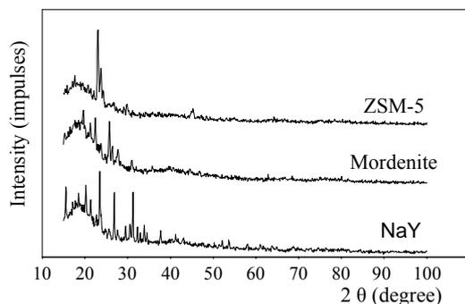
Fig.1 XRD of initial zeolites
