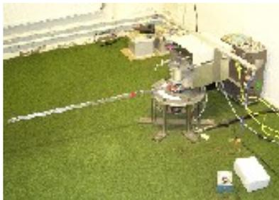
Fig. 1 The laboratory-scale single-link flexible manipulator
