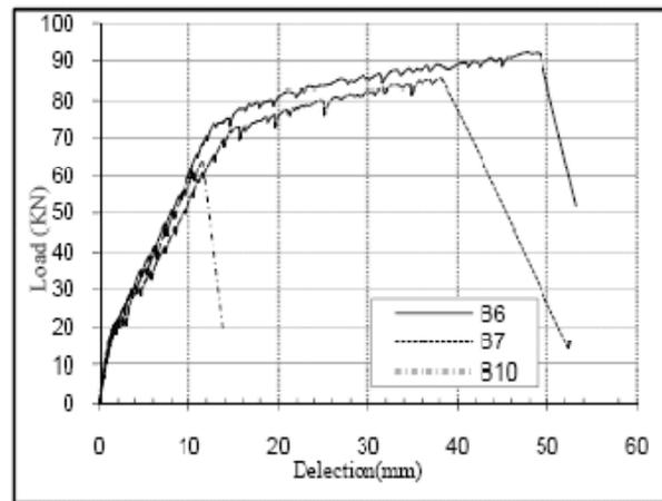
Fig. 9 Load-deflection curves for beam specimens with different lap splice length (vertical stirrups at 150 mm spacing in splice region)
