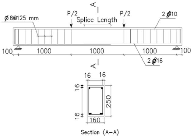
Fig. 1 Longitudinal and cross section details of beam specimens
