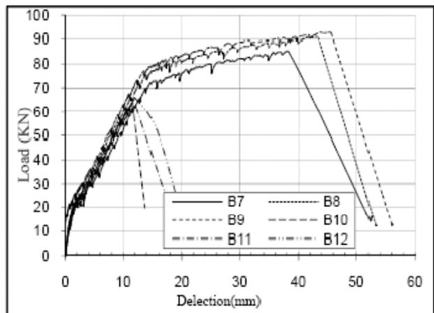
Fig. 10 Load-deflection curves for beam specimens with different vertical stirrups spacing in splice region
