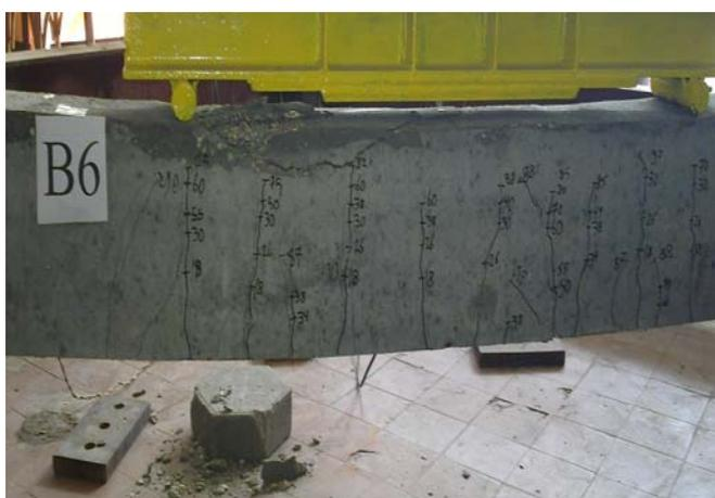
Fig. 7 Typical flexure failure for beam specimens
