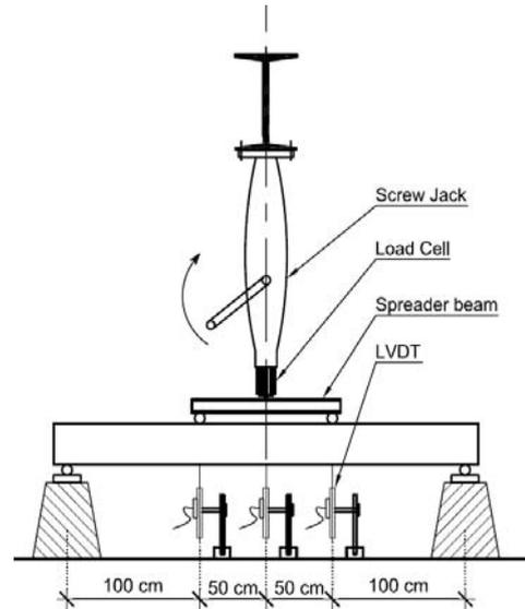
Fig. 3 Schematic of test set-up for splice beam
