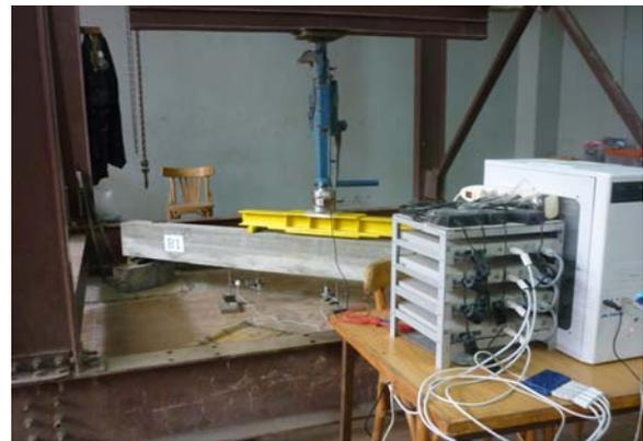
Fig. 4 Splice beam prior to testing
