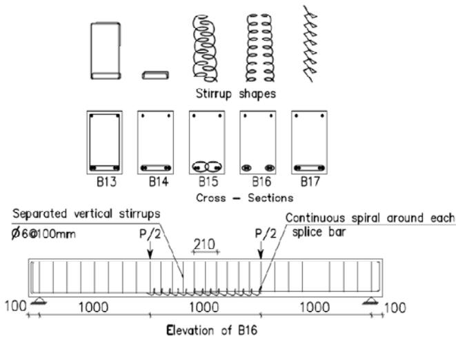
Fig. 2 Details of stirrups around spliced bars
