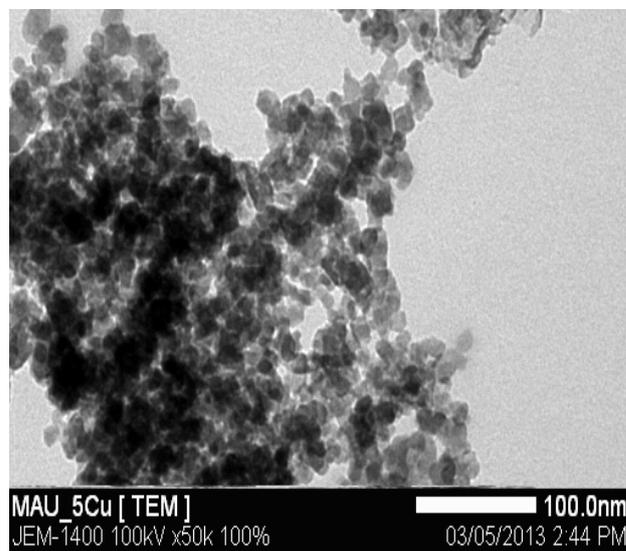
Fig. 2 TEM image of bimetallic Fe/Cu nanoparticles with Cu to Fe ratio of 1:20
