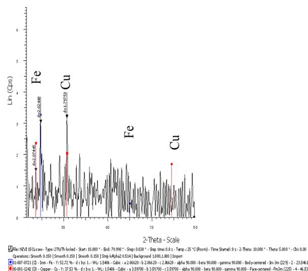
Fig. 6 XRD peaks of bimetallic Fe/Cu nanoparticles Cu to Fe ratio of 1:6.7
