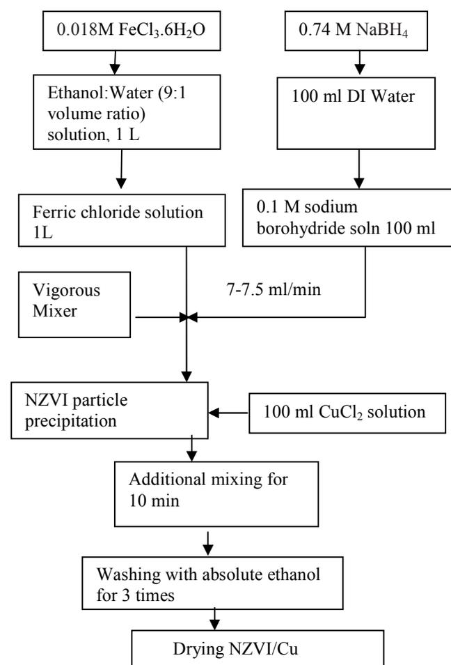
Fig. 1 Flowchart of Synthesis of Bimetallic Fe/Cu Nanoparticles
