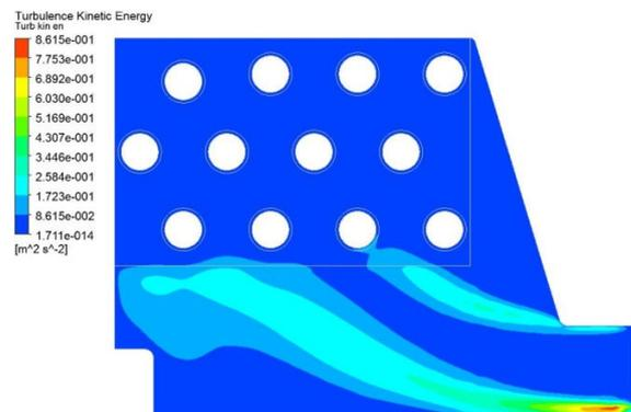
Fig. 10 Modeled turbulence kinetic energy
