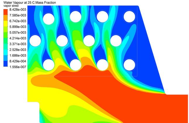
Fig. 8 Water vapor contours in middle plane
