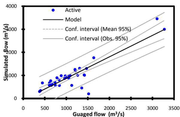
Fig. 6 Simulated versus observed monthly flow during the validation period (1993-1996)
