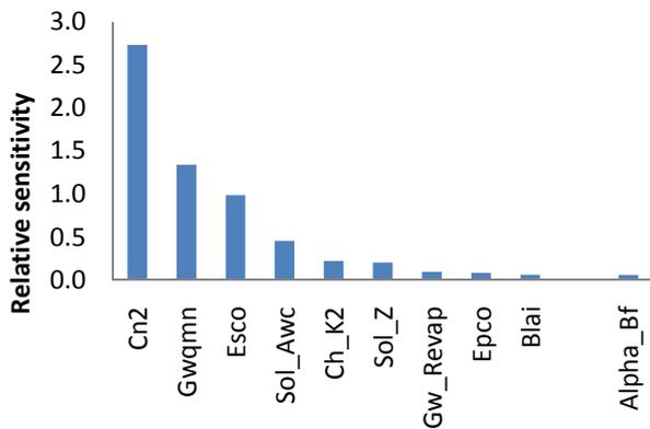
Fig. 3 Relative sensitivity and description of modeling parameters
