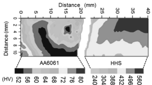
Fig. 4 Micro-hardness Profile of Bimetallic FSW Joint
