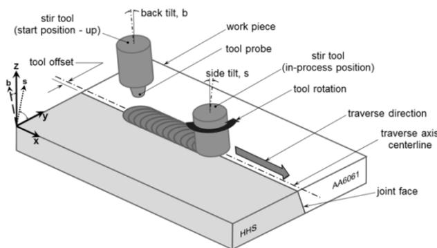
Fig. 1 Schematic of friction stir process and terminology
