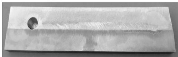
Fig. 2 Bimetallic FSW Coupon (top face milled)
