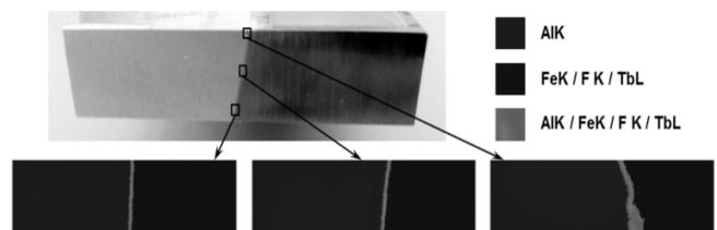
Fig. 6 Elemental Composition of Bimetallic FSW Joint
