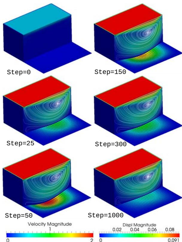
Fig. 8. Fluid Velocity, plate displacement and streamlines .
