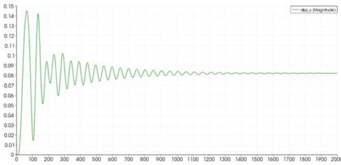
Fig. 4. Magnitude of the displacement at point 1.
