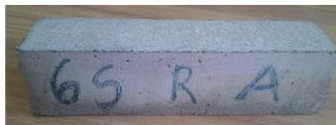
Fig. 8 PAG-10V specimen before the immersion in acid solution
