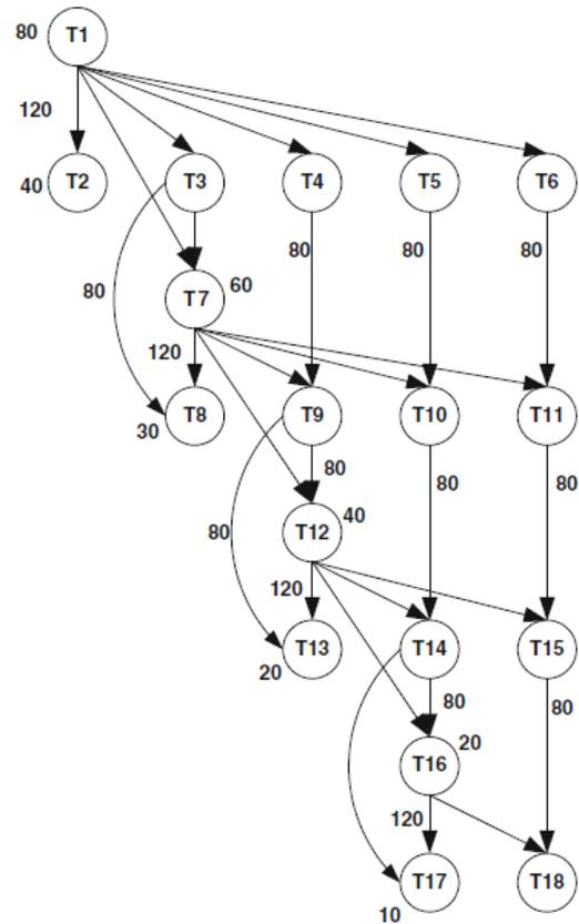
Fig. 1 Standard Gauss Elimination of 18 tasks & 4 processors [11], [13]
