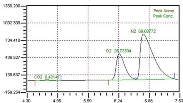
Fig. 5 Composition of gases separated from water
