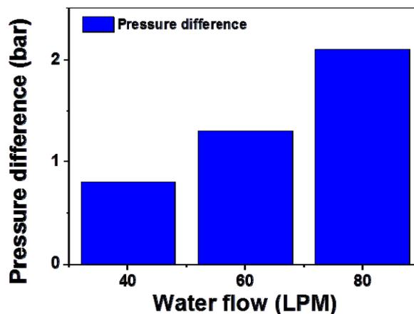
Fig. 6 Pressure drop for different water flows
