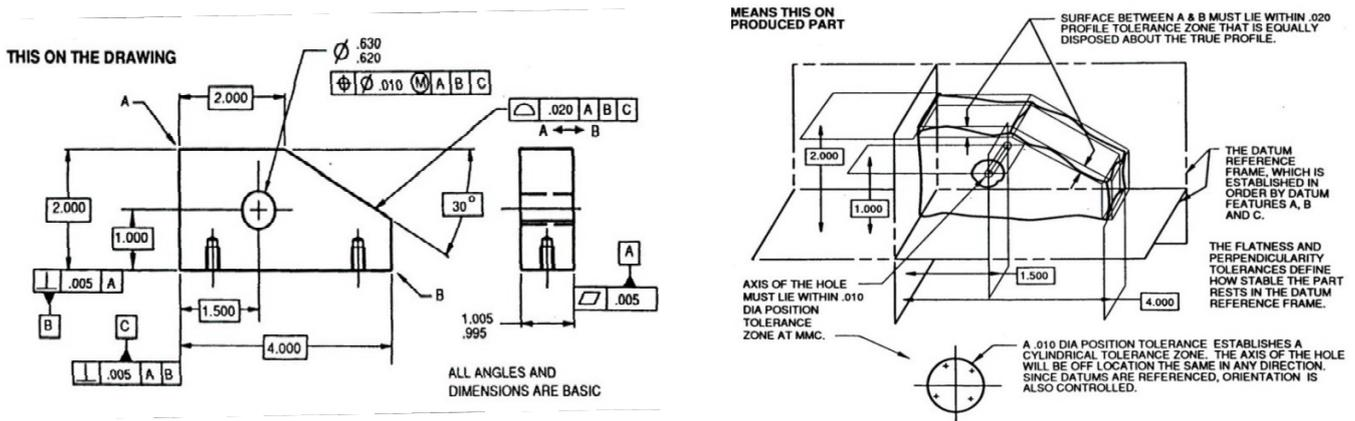
Fig. 2 GD&T applied to a simple angle block [9]
