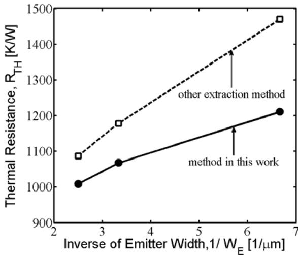
Fig. 3. Extracted thermal resistance  $R_{TH}$  as a function of emitter width (with constant emitter length  $L_E = 1.0 \mu\text{m}$ ) using the method described in this work (solid line with closed symbols) and verification using an alternative extraction method in [4] (dashed line with open symbols). We observe that the extraction method suggested in [4] over estimates the extracted  $R_{TH}$ , since it ignores the influence of collector-base Early effect on  $V_{BEi}$ .
