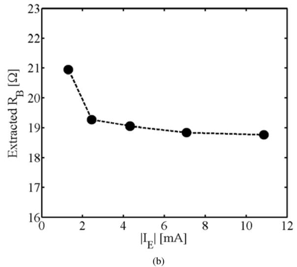
Fig. 2. Extraction of  $R_B$  and  $R_{TH}$  using the vertical intercept and slope of (3) for a device with  $A_E = 0.40 \mu\text{m} \times 1.0 \mu\text{m}$ . (a) Plot of  $-dV_{BE}/dI_C$  as a function of  $(V_{CB} + V_A^{eff})$  and  $I_E$  [measurements (symbols) and linear fits (dashed lines)]. (b) Extracted  $R_B$  (from vertical intercept of Fig. 2a) as a function of  $|I_E|$ . From the corresponding slope  $S_{TOT}$ ,  $R_{TH}$  is extracted.
