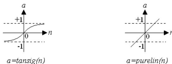
Fig. 3 Transfer functions for feed forward Neural Network
